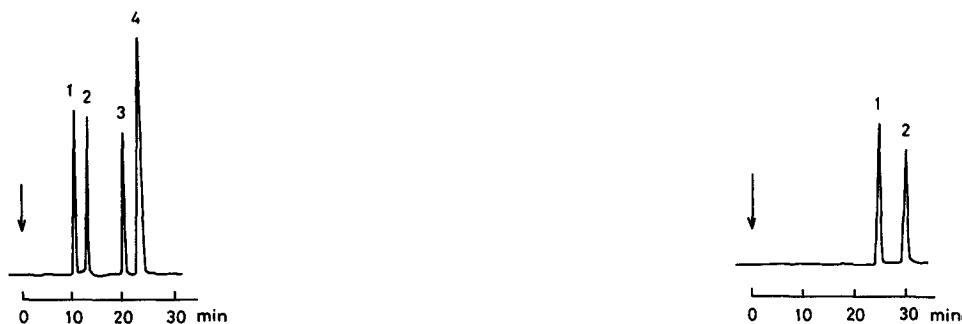
Fig. 2. Separation of a mixture of digitoxin, gitoxin, gitaloxin and internal standard I. Peaks: 1 = gitoxin; 2 = gitaloxin; 3 = digitoxin; 4 = 14\alpha,15\alpha -epoxy- \beta -anhydrodigitoxin. Conditions: Chemcosorb 5 C 8 -U column (150 mm \times 4.6 mm I.D.); mobile phase, acetonitrile-methanol-water (4:4:5); flow-rate, 0.5 ml/min; UV monitor at 220 nm; sample volume, 10 \mu l.
